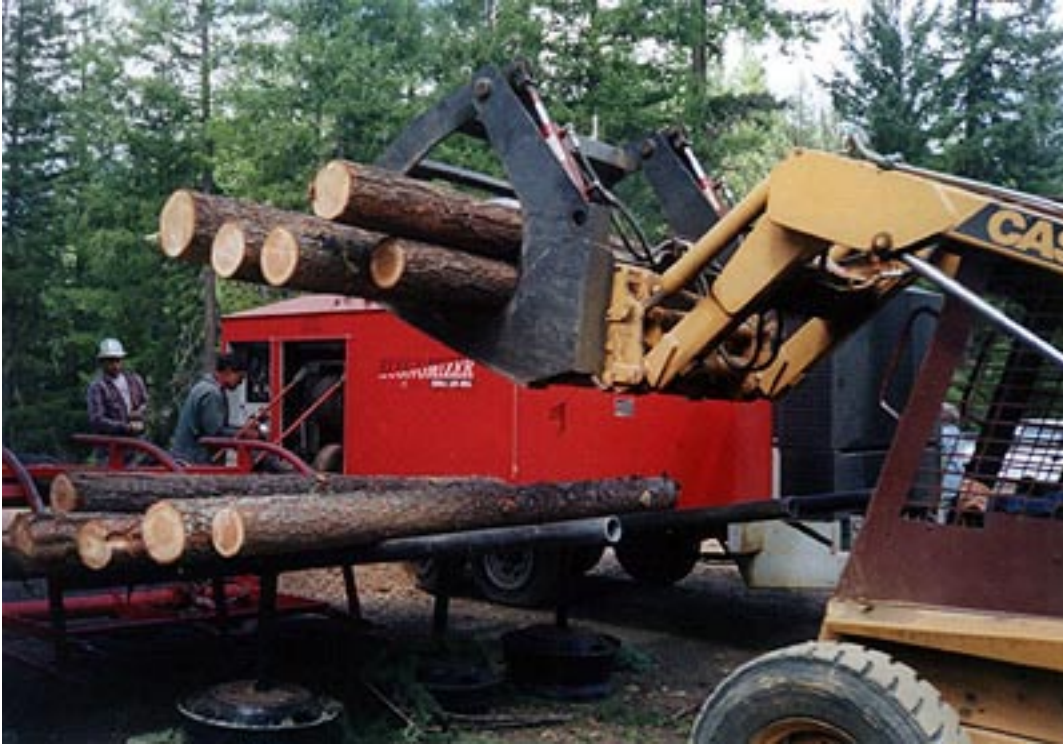
Small diameter timber processor used for milling lumber on-site
