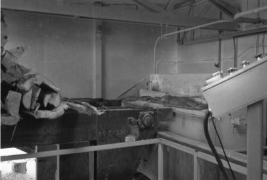
Machine that shreds juniper for pet bedding and other uses. REACH, Inc.
